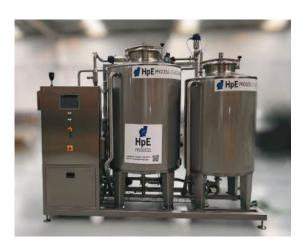
A typical system will include an installation tank, CIP send tank, CIP return pump, dosing pump, heating coil, butterfly valves (manual or automatic) and a control panel.
