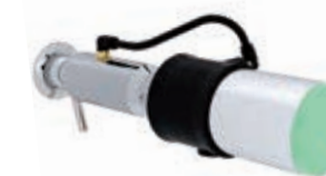
Pneumatic actuator, normally closed, equipped with a 24 VDC control head, with a single-acting solenoid valve and 2 limit switches (top and bottom) (Non-ATEX zone).
