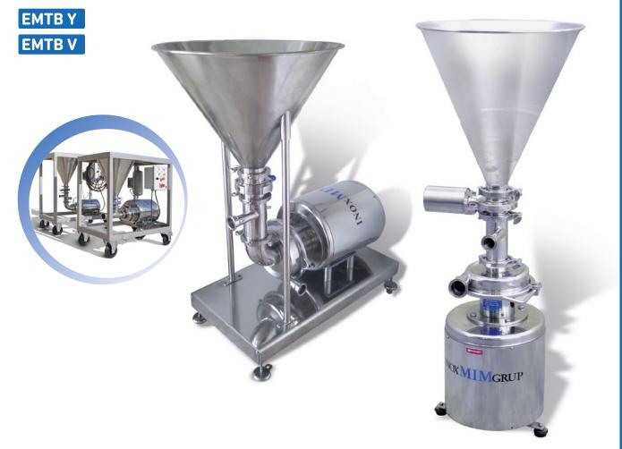
EMTB solid-liquid mixers, with the optimised design of the blade and suction system, produce completely homogenised mixtures of powders or granulated products with liquids. The simplicity of the parts and the connections system facilitate maintenance tasks and ensure highly hygienic operation conditions.
