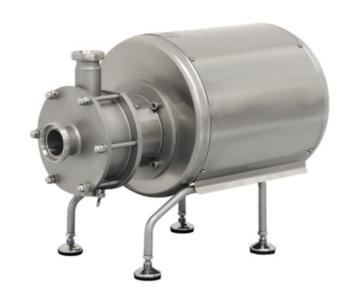
EML -- -- inline mixers provide high emulsion grades and are able to pump the product thanks to their slotted head and propeller design. These mixers achieve a completely homogenised, lump-free product and prevent oxidation. With the careful treatment they provide, they are highly recommended for handling and decanting already homogenised products, thanks to their ability to maintain the properties of the product whilst pumping.
