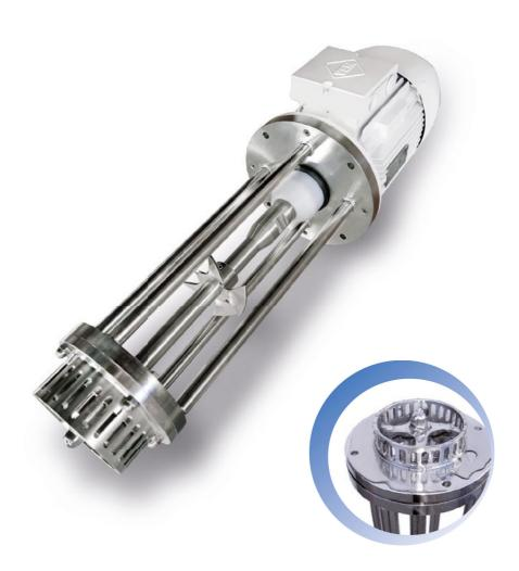
EM---- vertical mixers provide high shear rates in emulsions and dispersions due to their head and turbine design. The vertical mixer produces a completely homogenized product, without lumps, in medium (5000 litres) and small volume applications. Furthermore, because of the careful treatment they provide, these mixers are very useful for keeping the compound properties of products which are already homogenised.
