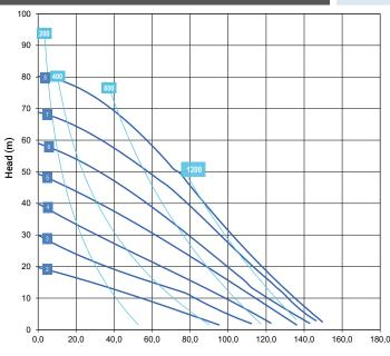
\* The curves and performances refer to pumps with submerged suction and free delivery outlet, with water at  $20^{\circ}\text{C}$  and vary according to the composition materials.
