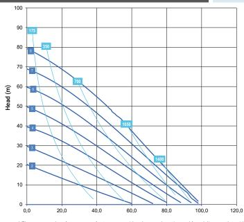
\* The curves and performances refer to pumps with submerged suction and free delivery outlet, with water at 20°C and vary according to the composition materials.
