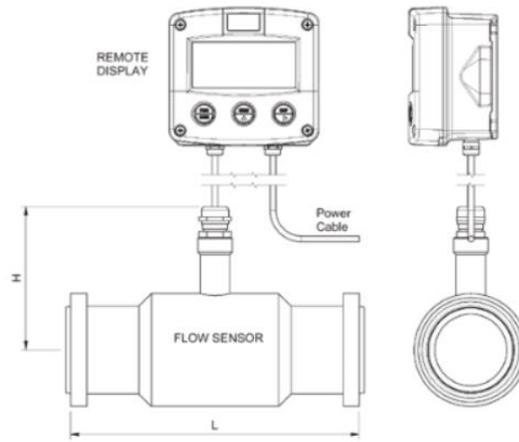
HBT Hygienic Turbine Flow Meter RJT Connections & Remote Display
