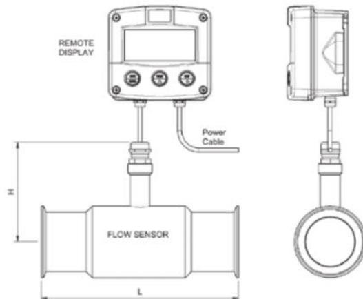
HBT Hygienic Turbine Flow Meter Tri Clover Connections & Remote Display
