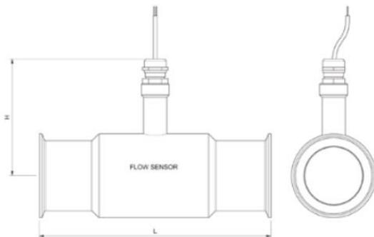
HBT Hygienic Turbine Flow Meter with Tri Clover Connections
