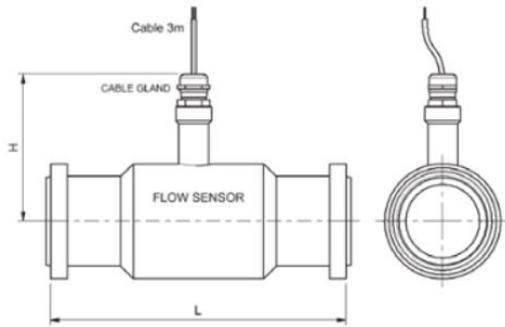
HBT Hygienic Turbine Flow Meter with RJT Connections
