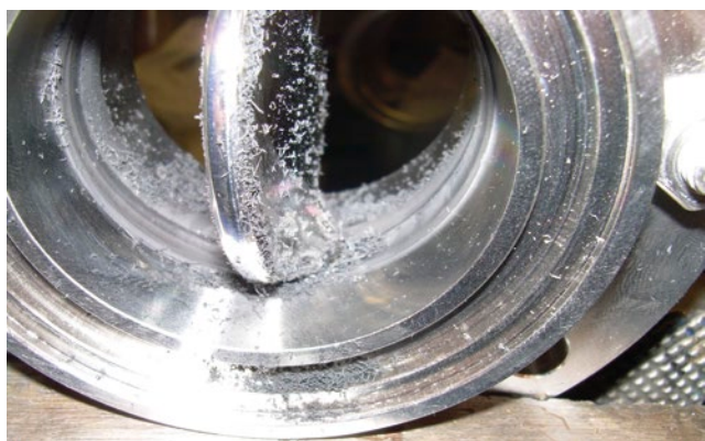
Figure 1. Seal abrasion at the disc.
