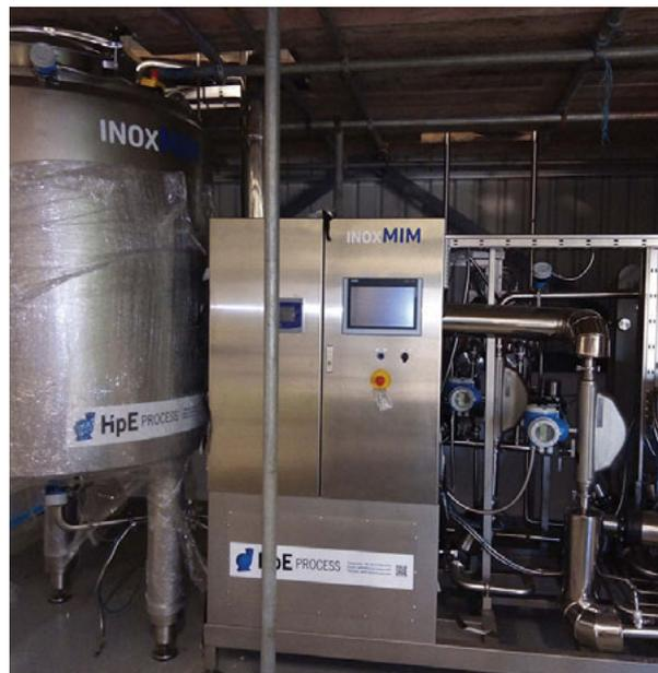
In the food industry it is important to demonstrate that the CIP has been done, so data logging collates information such as temperature, cleaning times and chemical concentration
